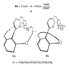
Two isomers of 10 are conceivable: (i) the concave bimacrocycle 10a and (ii) the bismetacyclophane 10b. CPK models and NOE-NMR experiments as well as protonation and complexation experiments support structure 10a.
